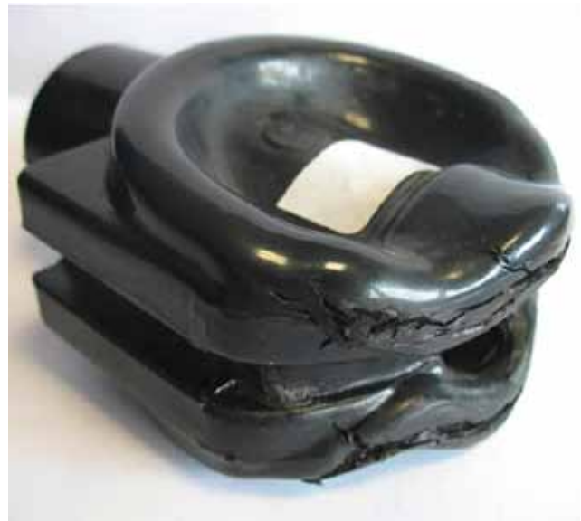
A critical feature of the RSGV is the wedge Poor design, process and manufacturing control lead to premature failure, affecting water quality and service levels.
